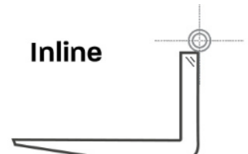
Inline The center of the eye is inline with the fork back
