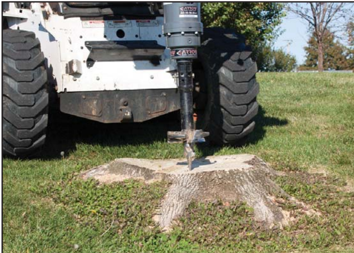
Blades make a clean, horizontal cut.
